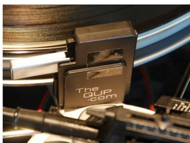
Test The Q UP with a few different records just to make sure it is working well for you. Once satisfied you can secure the position with a bit of transparent tape... if you like.
